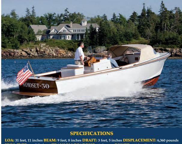
LOA: 31 feet, 11 inches BEAM: 9 feet, 8 inches DRAFT: 3 feet, 5 inches DISPLACEMENT: 6,360 pounds HULL TYPE: modified-vee TRANSOM DEADRISE: 18 degrees POWER: 440-hp diesel (prop or waterjet) SPEED: 49 mph top, 29 mph cruise PRICE: \$425,000 CONTACT: Samoset Boatworks, Boothbay, Maine. Phone: (207) 633-8350. www.samosetboatworks.com
